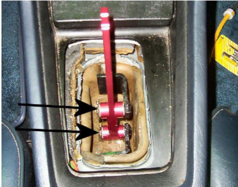
12. Once installed, put the retaining clips back on.
