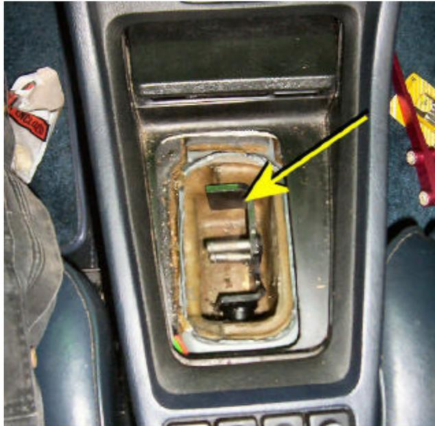
8. Good time to test the front shift cup for excessive play. Grab the forward shift rod and...
