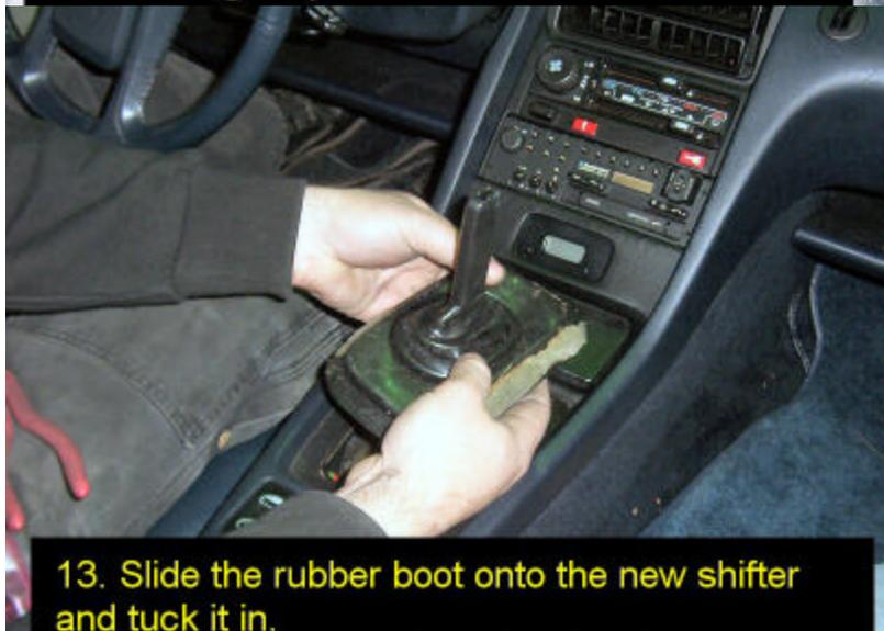
13. Slide the rubber boot onto the new shifter and tuck it in.
