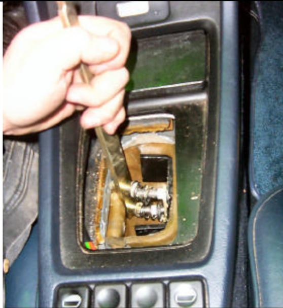
**6. Pull the old shifter off the end of the shift rods, and out.**
