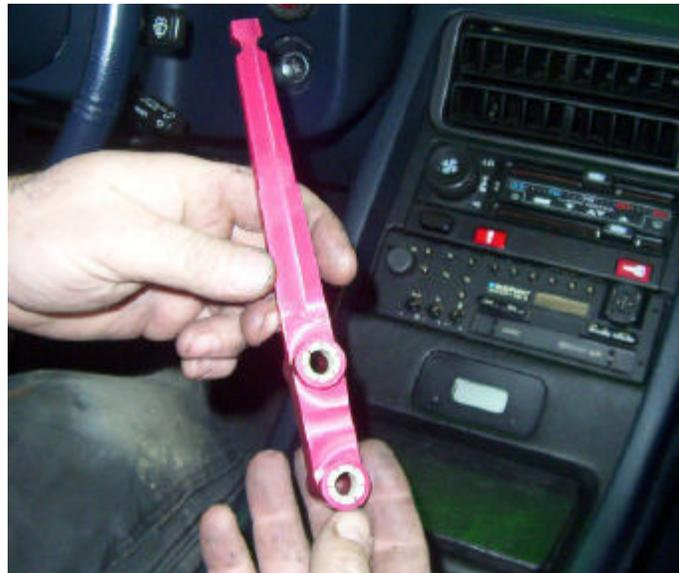
10. Place the nylon bushings in the new short-shift lever.
