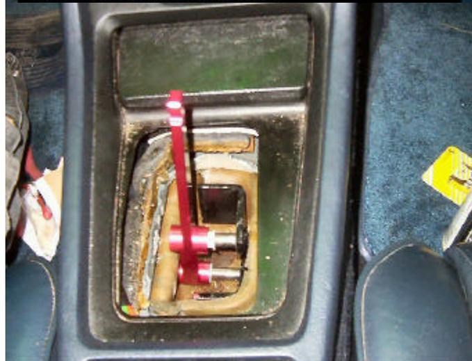
11. Slide the shift lever onto the shift rods as shown. Cleaning the old grease off the rods makes it easier.
