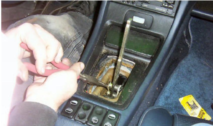
**5. Remove the retaining clips with a needle-nose pliers.**
